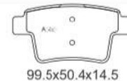
99.5x50.4x14.5 SYL-2226 Mondeo III 1.8i 16V, 1.8 Sci, 2.0i 16V, 2.5 V6 24V, 3.0 ST 220, 3.0 V6 24V 05> Tras. Sist. Bosch
